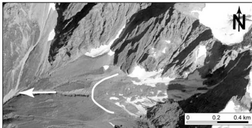
Figure 7. Area of initiation of the 2005 Rotlauri-Guttannen debris flow. The white line delineates the lower margin of a frozen body of glacial sediment. Remnants of Homaf Glacier are visible at the foot of the rock face at the right side of the photograph. The glacier formerly extended to the white line and left large amounts of sediment during its retreat. The sediment probably only became permanently frozen after retreat of the glacier. The arrow indicates the direction of debris flow propagation.
